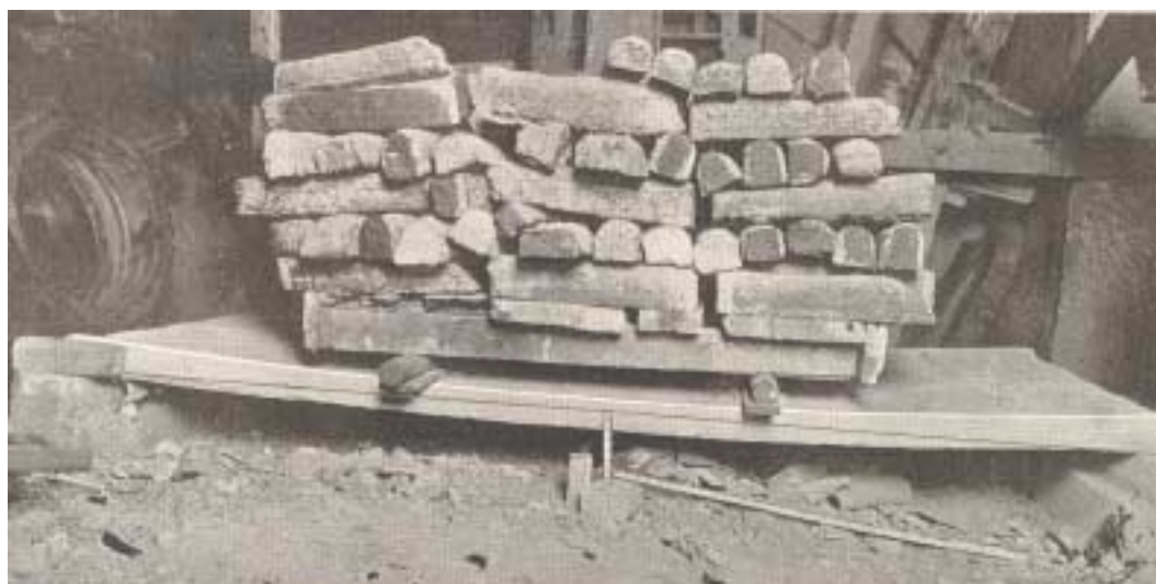
Figure 4. Test of “Gunite” slabs made under supervision of Prof. M. O. Fuller, Lehigh University. [The tests were started in 1920 and ran through 1934. The 8' 0" (2.4 m) span, 3-1/4" (82.6 mm) thick, deflected 2" (50 mm) by 1922 and stressed the reinforcing to 36,000 lb (160 kN) at completion. No further deflection occurred after the 3rd year.]
